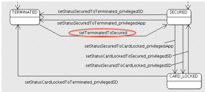
Figure 8. Example of a violating fragment of the GP 2.1.1 Life-Cycle modelled with ArgoUML
